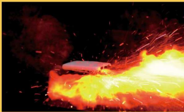
▲ Fire outbreak caused by mobile batteries or power banks (re-enactment experiment)
